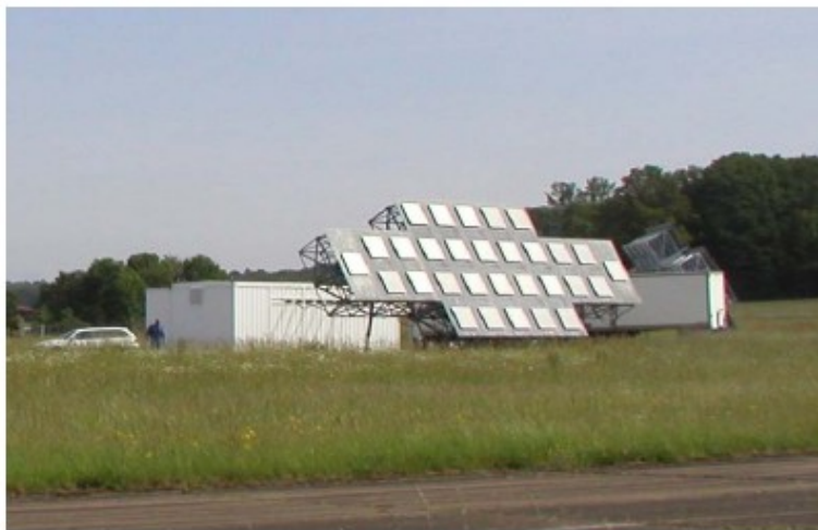
Figure 15 : transmitting array of patch antennas
