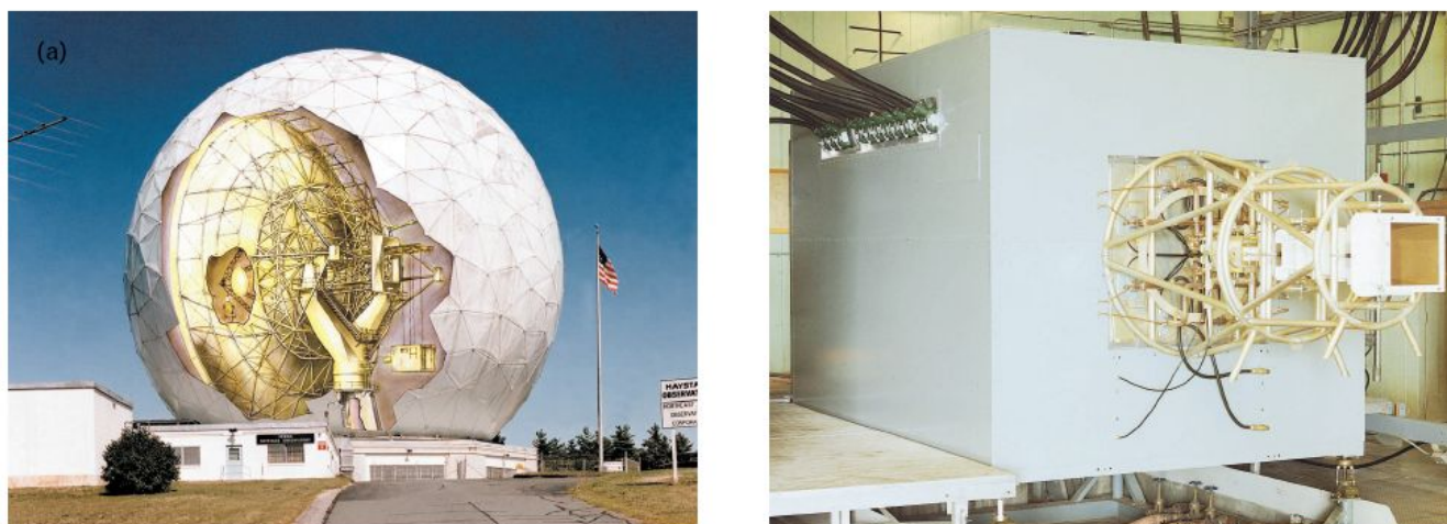
FIGURE 3. (a) Artist's rendition of the 120-foot Haystack antenna in its 150-foot radome; (b) the long-range imaging radar (LRIR) feed horn and transmitter/receiver radio-frequency (RF) box in its test dock in the Haystack radome.
