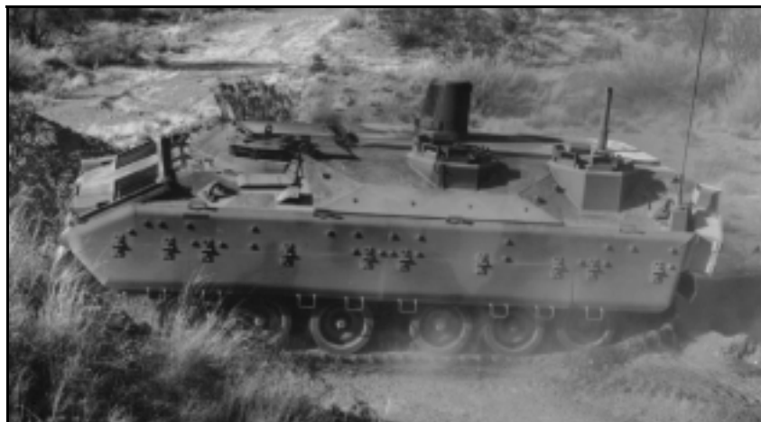
The shape of things to come? A missile-armed Future Combat System might resemble the Bradley-LASAT prototype shown here. A very low silhouette is made possible by a turretless configuration. (Photo: Loral Vought Systems)
