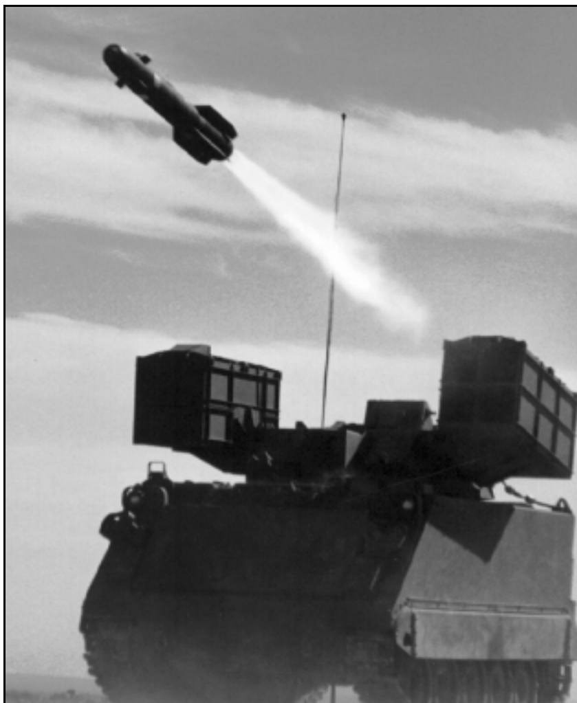
Hellfire, seen here being fired from an M113, can hit targets as far away as 8000 meters—almost three times as far as the Abrams! If adapted to the Longbow Hellfire system, ground forces would have a heretofore unknown combat capability. (Photo: Rockwell International)
