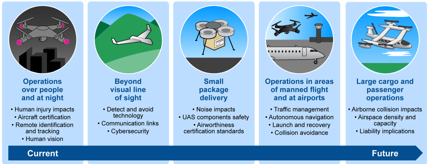
Figure 2: The Federal Aviation Administration’s Incremental Phases for Unmanned Aircraft Systems (UAS) Integration and Examples of Key Capabilities or Topics to Be Researched during Each Phase, as of October 2019
