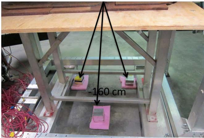
Figure 6) Set up used to mockup warhead counting with detectors above a missile hatch. The hatch was assumed to be about 1" of steel in thickness. The neutron detectors were on the floor, so were not shielded by the steel, but this is estimated to have a minimal effect on counting rates.
