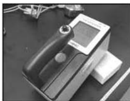
Figure 1.2: A handheld RIID. SOURCE: DND O (2008a)
