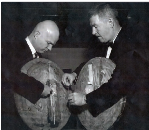
Figure 14: The Great Seal Bug. Director of Security John Reilly (right) holds the cavity resonator, and an SY Agent points to where the Soviet listening device (or “bug”) was placed in the wood carving, which hung in the U.S. Ambassador’s official residence in Moscow, Spaso House. SY technical officer Joseph Bezjian discovered the bug with the aid of Ambassador George F. Kennan, who read a published Department document while Bezjian located the origin of the frequency. Bezjian shipped the bug to Washington, and Secretary of State Dean Acheson showed it to President Harry Truman and explained how the bug worked. Truman ordered U.S. Government agencies to develop countermeasures for such technological espionage. Source: Department of State Records, National Archives and Records Administration.
