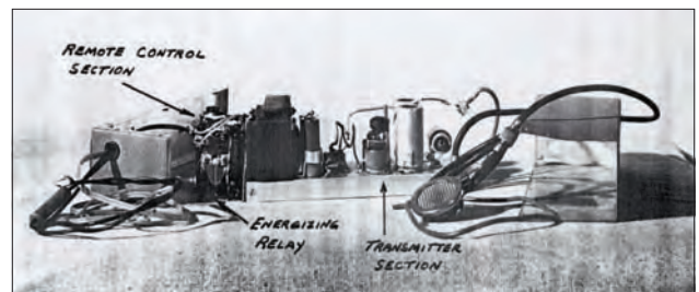
Figure 15: SY technical engineers found this listening device in the U.S. Embassy in Prague in 1954. During the early years of the Cold War, SY found many listening devices in U. S. Embassies in Soviet bloc countries. In fact, between 1948 and 1961, SY engineers discovered more than 95 percent of all listening devices found by all U.S. Government agencies. Source: Bureau of Diplomatic Security Files.
