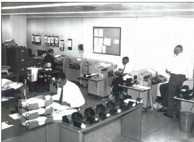
Figure 9: The Department of State's Communications Center as it appeared in October 1961. Although the Department had adopted Telex printers, much of the Department's equipment relied upon World War II technology. Delays in receiving telegrams were common because Department telegram traffic had risen sharply since 1945. Source: Department of State Records, National Archives and Records Administration.
